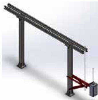
Earthing switch structure
