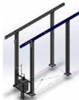
Disconnecting switch structure
