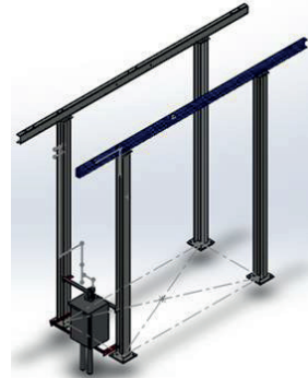
Disconnecting switch structure
